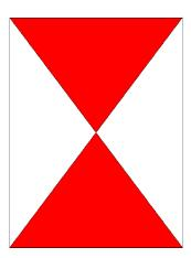
The plates shall be on the same height above buffer on the transversal axis
