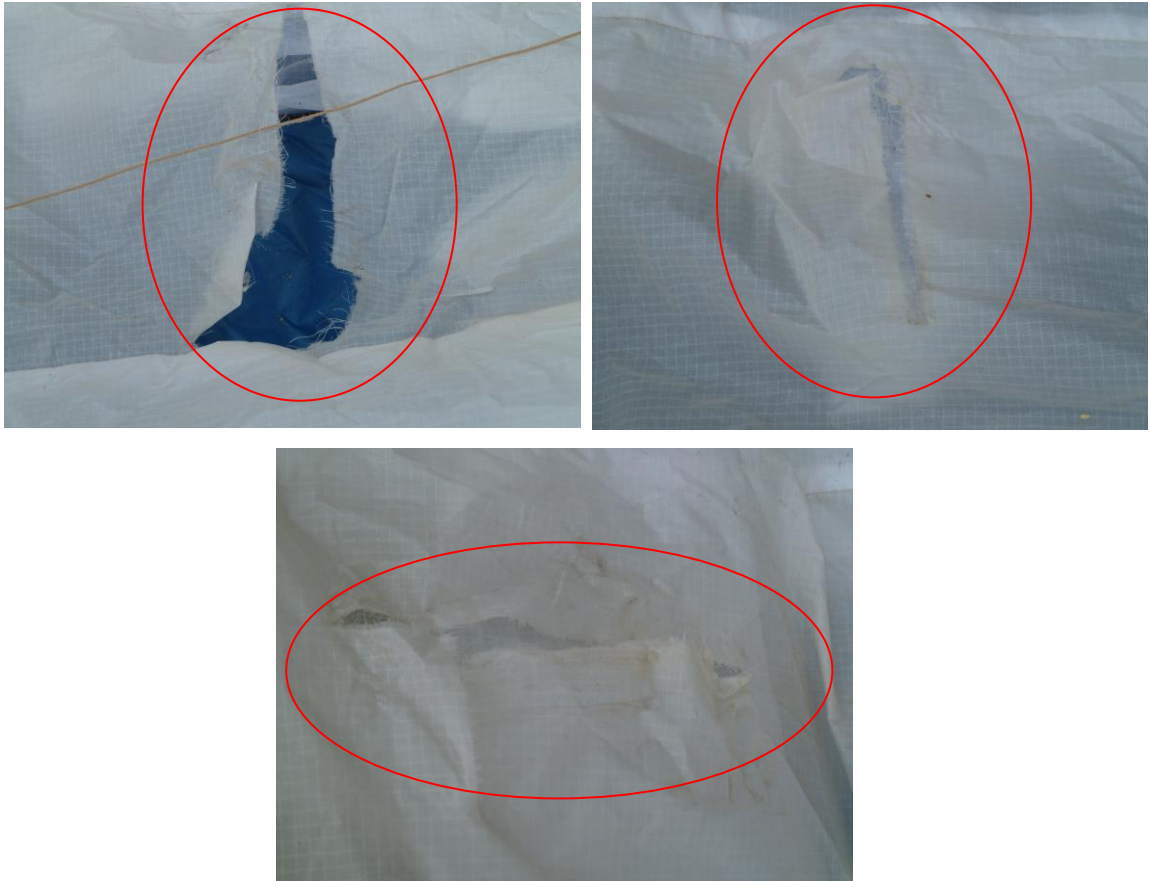
Fig. No. 3 Damage to the chamber of the PG canopy after the impact on obstacles
