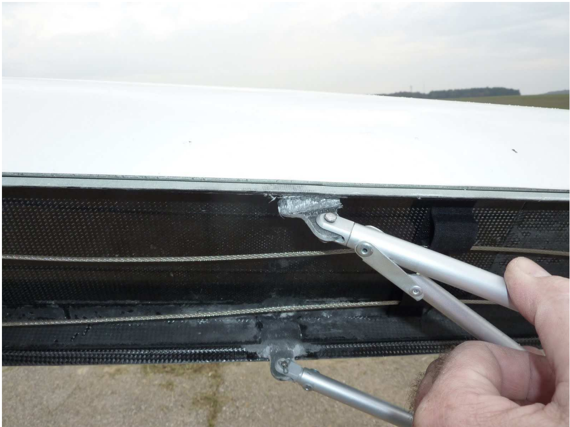
Fig. 3: Damaged upper attachment of Phantom PHG wing rib
