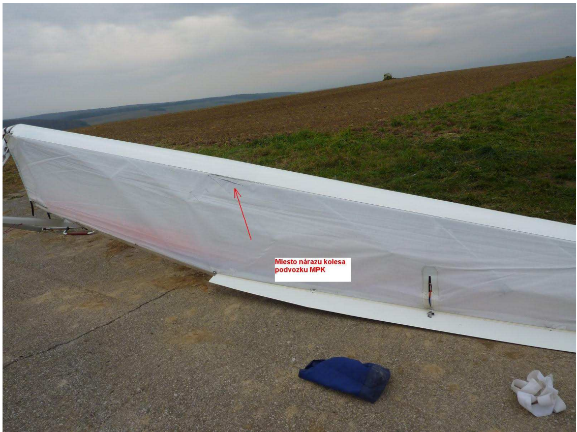
Fig. 1: Wing of Phantom PHG and point of impact of the landing gear wheel
