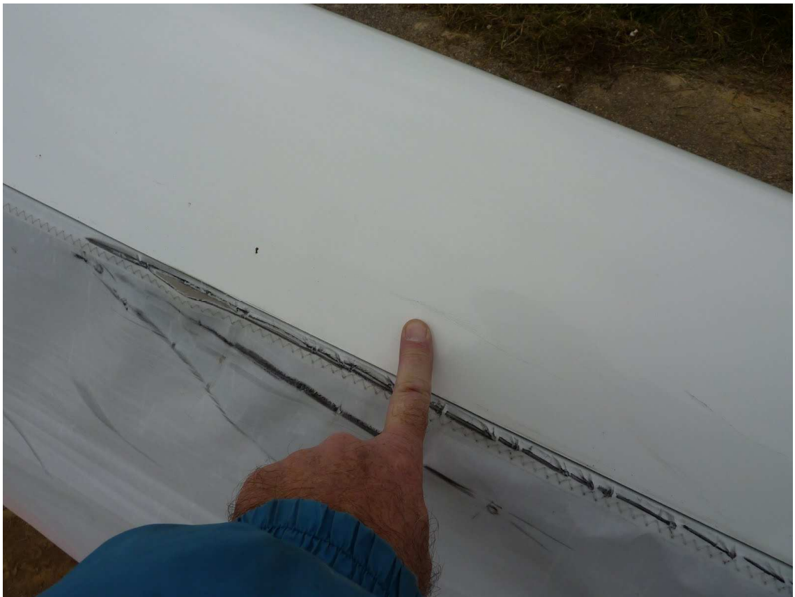
Fig.. 2: Damaged D-box and wing covering of Phantom PHG
