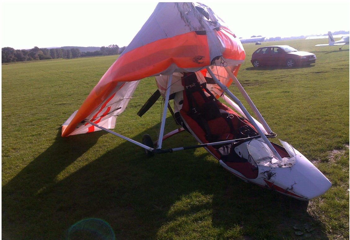
Fig. 1: Damaged PHG (picture taken after PHG positioning on landing gear wheels)
