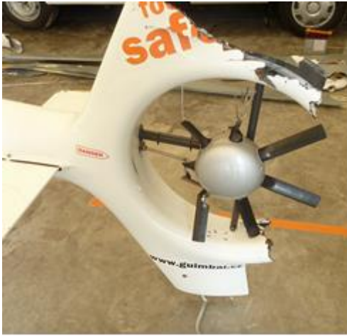
Pictures 1, 2. When the helicopter fell down, the fenestron and consequently the MR and the engine were stopped by force
