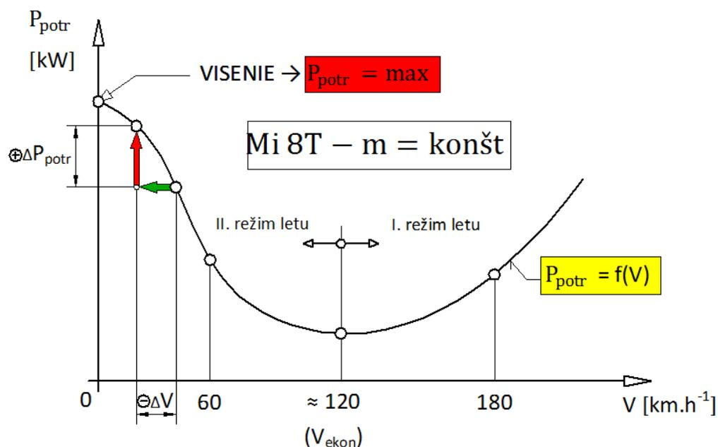
Besides the flight mass and flight speed, concrete values of required input depend on the flight height, air temperature and air humidity.
