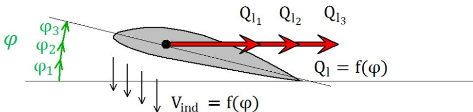
At a larger angle of adjustment of MR blades the induced air speed under the rotor  $V_{\text{ind}}$  and hence the thrust of PR, which brakes the descent of the helicopter, increase. However, the aerodynamic resistance of blades  $Q_1$  and hence the moment of aerodynamic resistance of MR blades against rotation, which has the effort to brake the rotational speed of PR, increase as well.
