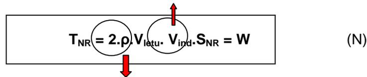
When decreasing the flight speed  $V_{\text{flight}}$ , the pilot has to increase the induced speed  $V_{\text{ind}}$  of air mass accelerated by MR in order to maintain the required thrust of MR  $T_{PR} = W$  and the possibility of control with the aim to maintain a sufficiently low speed of vertical descent with approach to the ground (in the final phase approx.  $0.2 \text{ m.s}^{-1}$ ). This process requires the increase of the angle of collective adjustment of MR blades  $\varphi$ .
