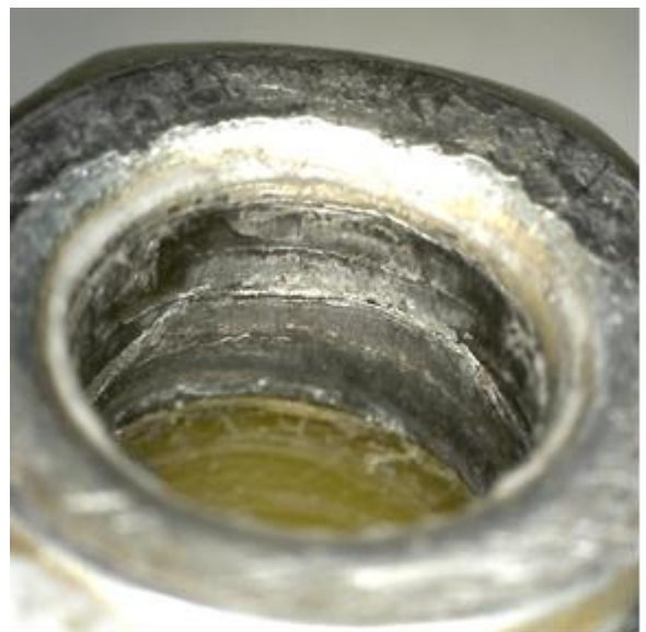
"Smoothed" internal nut thread
