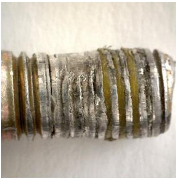
Detail view of the damaged bolt thread
