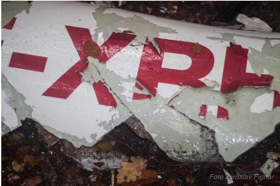
Fig. 17 Fragment of the coating with registration details
