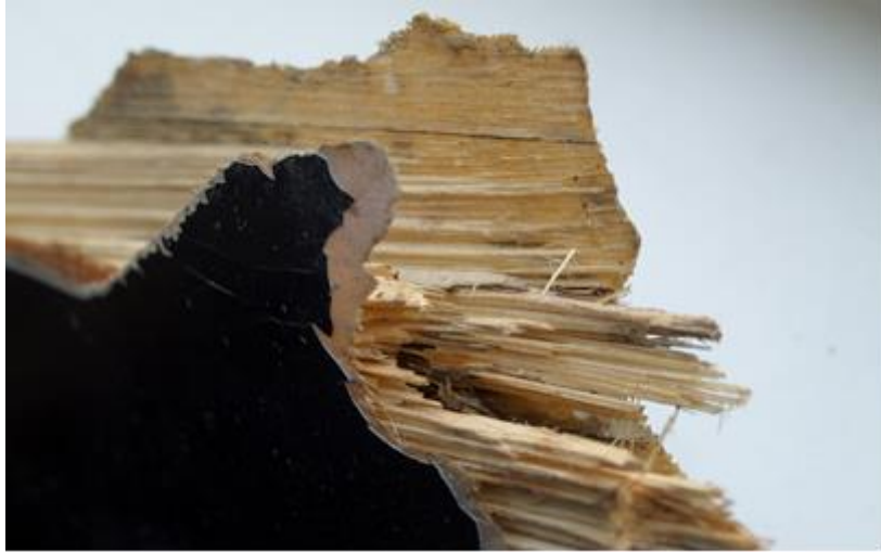
Fig. 25 Significant longitudinal cracks and missing material in the rear of the propeller blade
