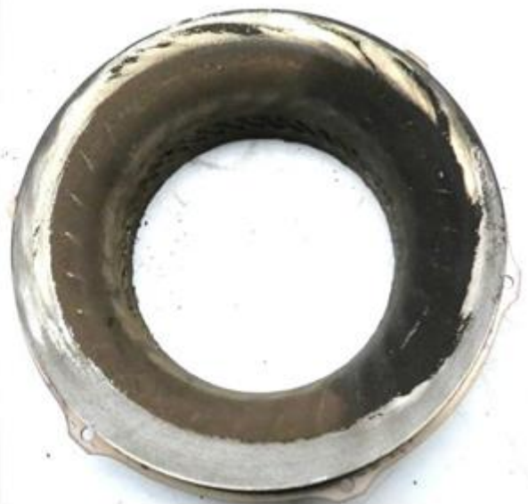
Ring of the rotor mast in the direction of the current, with friction marks (arrows)
