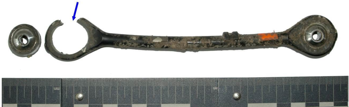
Damaged rod of the rear rotor blade mechanism
