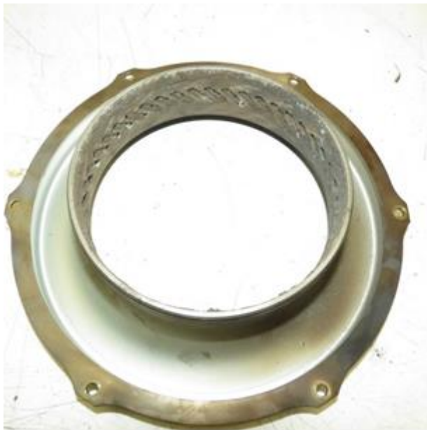
Ring of the rotor mast against the direction of the current, clay deposits (arrows)
