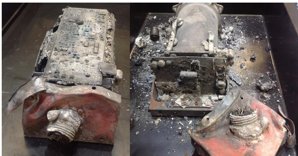
The outer layers were stripped from the device, and four broken memory chips were selected (CVR 1, CVR 2, FDR 1 and FDR 2)
