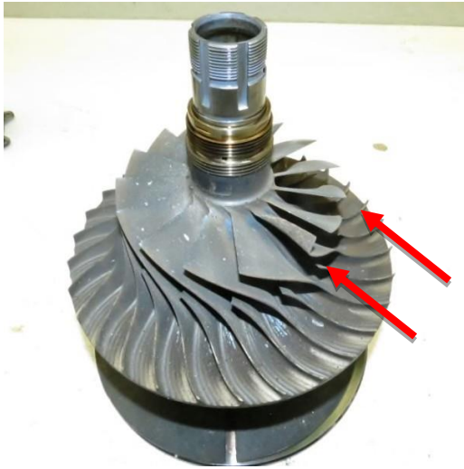
Rotor mast, bent blades (arrows)
