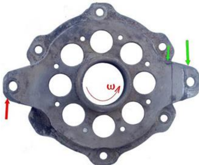
Input flange of the input flexible coupling of the right-hand drive shaft – the arrows indicate the edges damaged by the impact of the flange into the fixed obstacle
