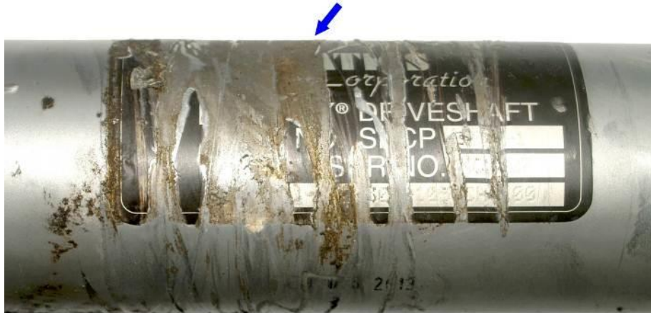
Circumferential scratching showing shaft rotation at the time of the emergency
