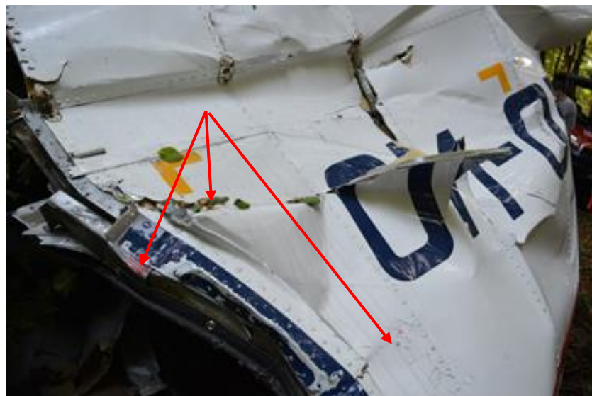
Traces of red colour on OM-ODQ from the wingtip arc of OM-SAB
