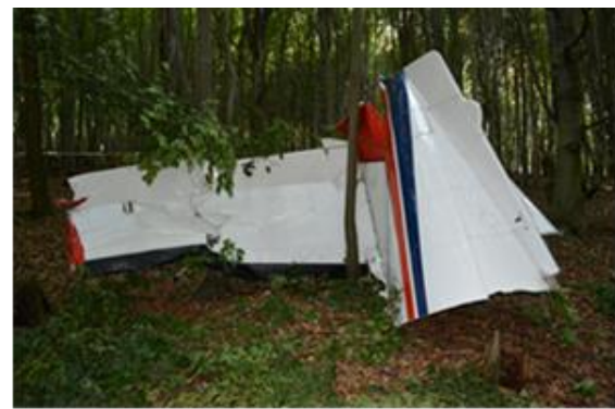
Separated tail of OM-ODQ near the 24 th partition
