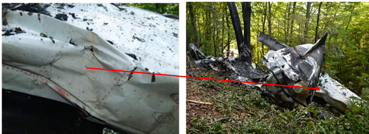
Damaged part of the right horizontal tail surface of OM-SAB from separated tail of OM-ODQ
