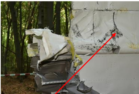
Traces left by aircraft OM-SAB on the separated tail of OM-ODQ
