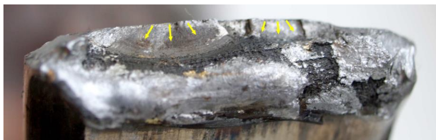
Photo No. 3 Mirror image of rupture on the connecting rod shaft
