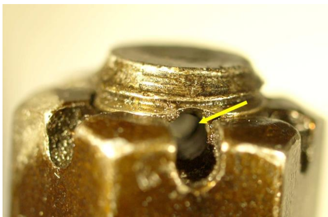
Photo No.6 Missing safety pin on crown nut
