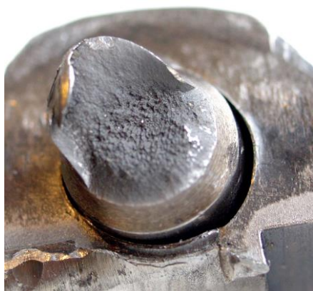
Photo No. 5 Rupture of connecting rod screw
