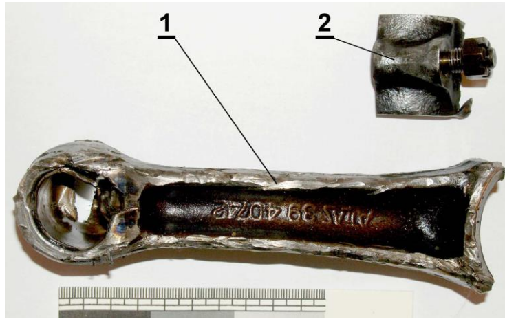
Photo No.1 Submitted parts of damaged connecting rod
