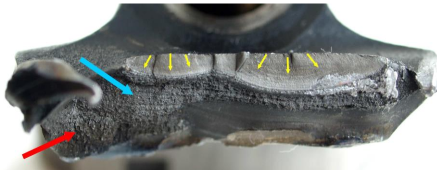
Photo No. 2 Visible fatigue rupture on the fragment of connecting rod head
