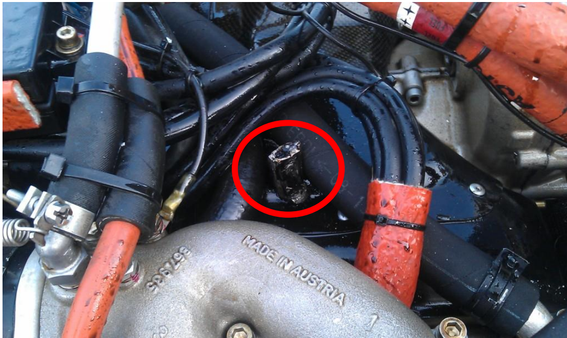
Fig. 3 Punctured engine block, fragment of connecting bar No 3 of the engine cylinder
