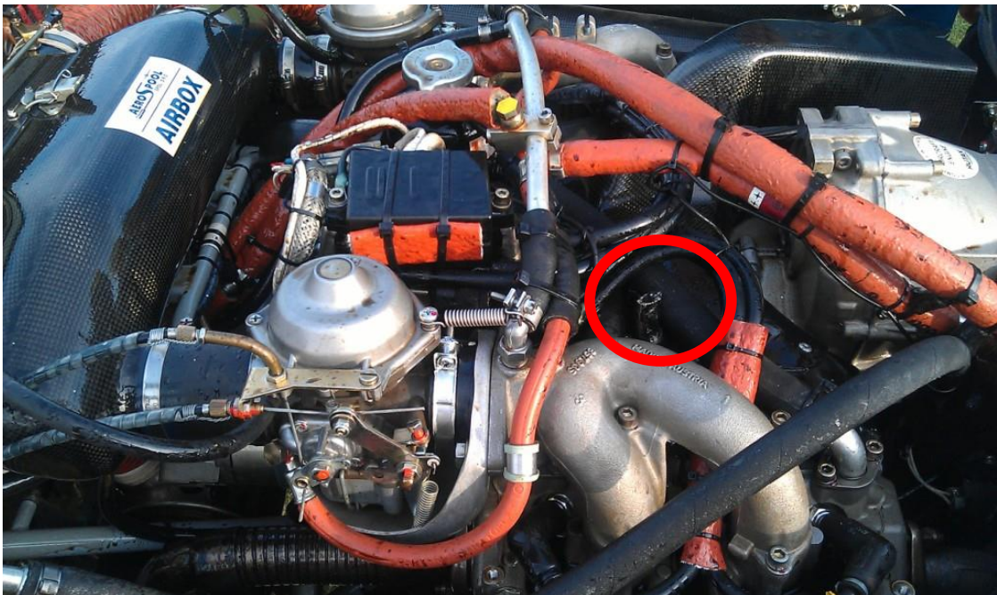
Fig. 2 Punctured engine block
