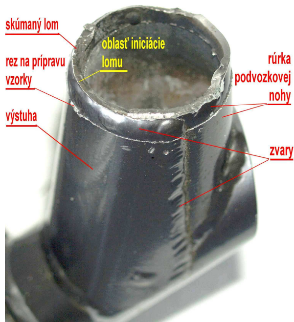
Fracture initiation area in the lower part of damaged landing-gear leg cross-section
