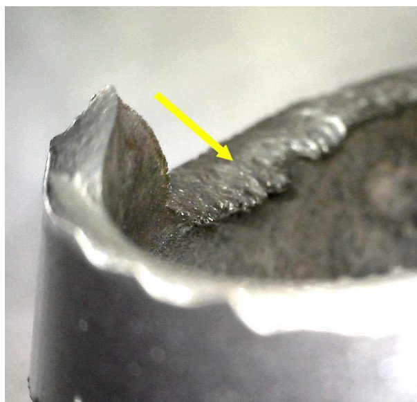
Bruising of the fracture surface in the area "C"
