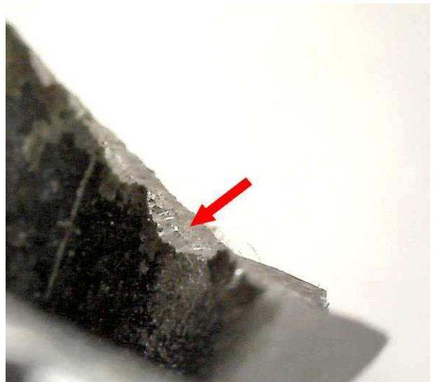
Deformation of the fracture surface margin in the area "D" inwards into the tube
