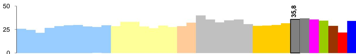
**STATIC MODULUS OF ELASTICITY OF CONCRETE IN COMPRESSION ACC. TO ISO 6784 (GPa)**
