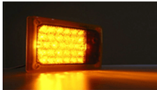
LED light unit consisting of some 30 LED's
